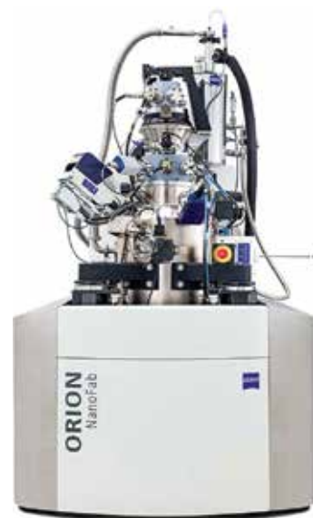
The Florida Institute for Cybersecurity Research's nanoscale imaging instrument can detect potentially malicious tampering in chips.
